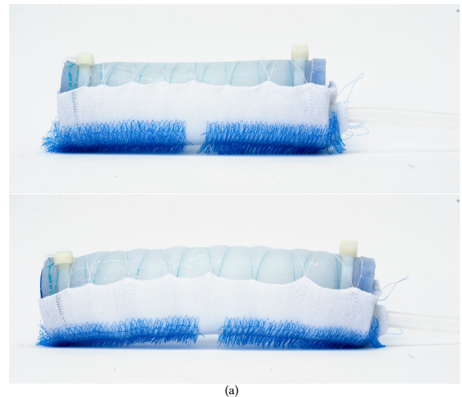
Figure 12: Biased bristles as cladding on a pneumatic extension actuator.
