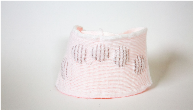
Figure 15: The soft control pad from Figure 1. Different thickness provide tactile cues to the location of capacitive button traces.
