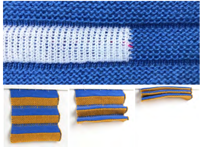
Figure 19: Using areas of differing knit/purl patterns to form a hinge or pleat. Top: A sheet with a pocket, which is part of the lamp example 28. The blue area is a single layer of knitting, primarily garter stitch, and the white is a second layer that connects to the blue layer at the top, bottom, and right edge, forming a pocket. Just above and below the pocket, full rows of all-knits define pleats that will bend forward (valley fold). Bottom: hinge areas allow the active position of a sheet-shaped sample to fold along pleat lines.
