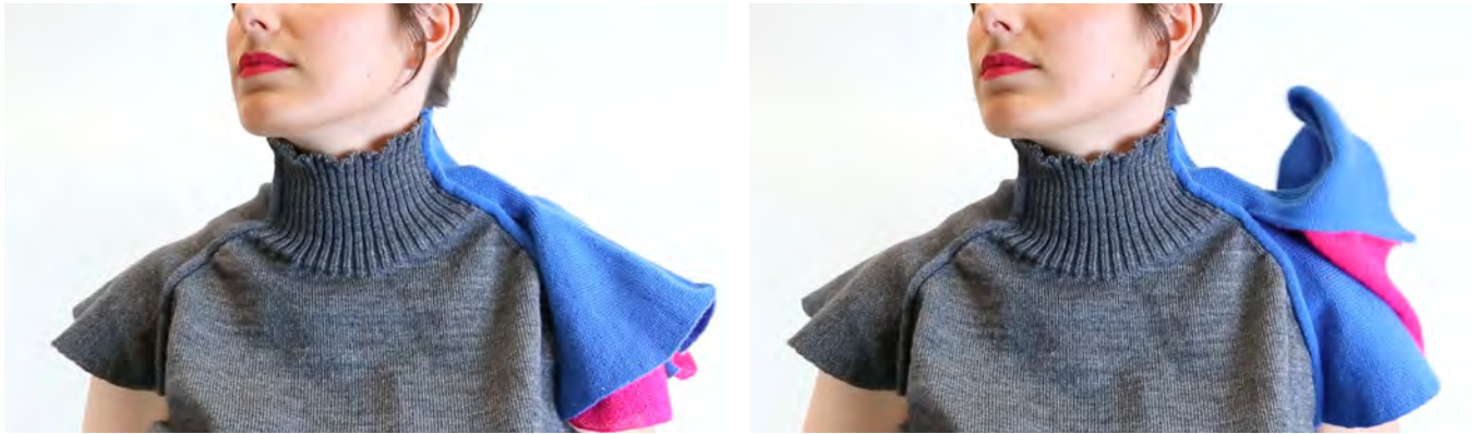
Figure 29: A sweater with actuated sleeve.
