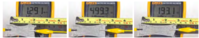
Figure 23: A swatch knit with Bekaert 50/2 Cotton plated with a hair-thin latex elastic, shown at 0%, 25%, and 50% stretch.
