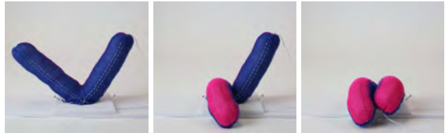
Figure 8: A horizontal tube with inlaid tendon and decrease shaping to bend the tube into a v-shape.
