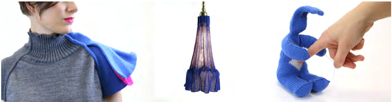
Figure 1: Left: a sweater with actuated sleeve. Center: a reconfigurable lampshade. Right: a responsive plush toy. These objects have been machine-knit using a collection of techniques discussed in this paper, such as shape and stiffness manipulation, combined with integrated tendon actuation.
