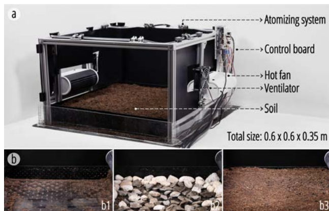
Figure 11. Testing chamber setup. (a) The chamber consists of an atomizing system, an electronic control, and hot air circulation above the soil. (b) Arrangement of cobblestones and fiber soil.
