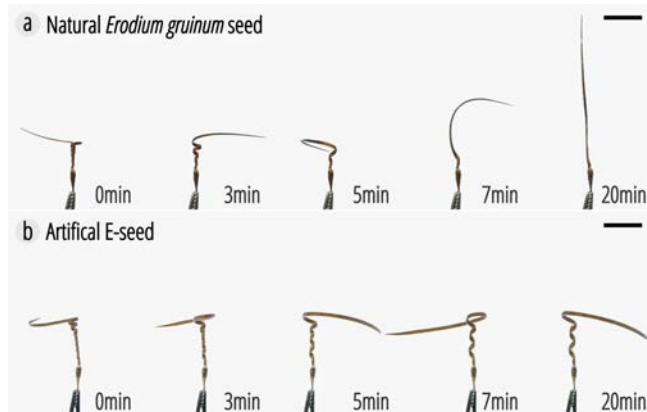
Figure 2. Comparison of (a) Erodium gruinum seed and (b) our E-seed undergoing a hydration process. Scale bar: 20 mm.
