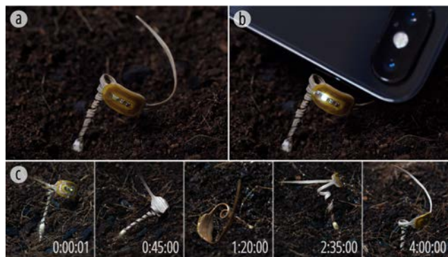
Figure 15. (a) E-seed carrying the RFID tag establishes itself in the soil. (b) E-seed responds to the cell phone NFC reader to light up an LED. (c) RFID attached E-seed established in 4 cycles.
