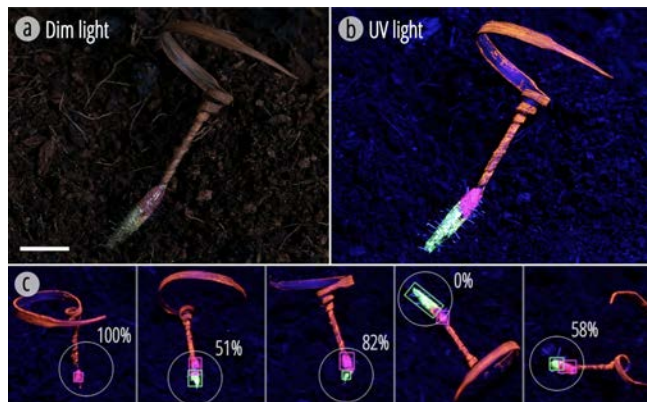
Figure 14. Fluorescent E-seed for vision-based remote monitoring under (a) poor ambient light, and (b) UV light at night. (c) Identifying tip burying percentage by a customized image processing tool. Scale bar: 10 mm.
