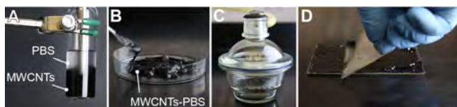
Figure 5. The preparation process of MWCNTs-PBS sheets.
