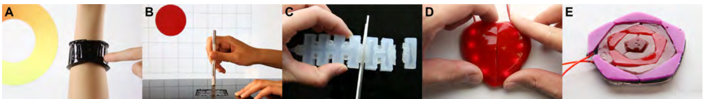
Figure 1. Application examples. (A) A transformative soft controller. (B) A Conformable damage sensor matrix. (C) A reconfigurable pneumatic actuators. (D) A self-healing heart with embedded LEDs. (E) A fusible, color-changing rose puzzle.
