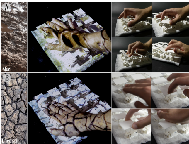
Figure 14: Interacting with the kinematic material display, simulating (A) mud with four DOF and (B) stiff dried soil with 2 DOF.
