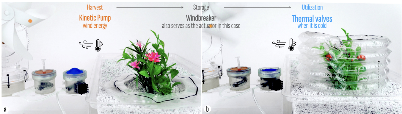
Figure 1: An example Sustainflatable system which can perform self-regulating plant insulation. The wind energy is harvested through a wind pump. The thermal valves incorporated in the system can sense the ambient temperature and adjust the inflation of the windbreaker accordingly. During warm weather, the windbreaker remains deflated (a). In contrast, during cold and windy weather, the system utilizes the collected energy to inflate the windbreaker and provide insulation to the plants (b).
